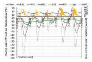
Fig. 4 The data obtained computationally for heat flow response corresponding to the cooling energy load for vented test case (*Note EXP* results obtained for unvented test case)
