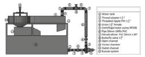
Fig. 4 Experimental Setup for laboratory work
