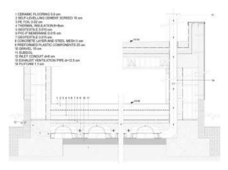
Fig. 5 Air gap with igloos and exhaust vertical ventilation pipe
