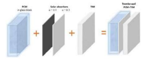
Fig. 1 Material combination of thermo-physical advances in Trombe wall
