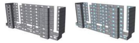
Fig. 4 Geometrical discretization of facades for concrete (left) and timber panels (right)
