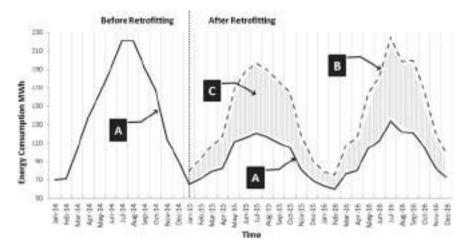
Fig. 1 Building energy consumption before and after retrofitting.  $\mathbf{a}$  is actual consumption.  $\mathbf{b}$  is estimated consumption if there was no retrofitting.  $\mathbf{c}$  is the estimated saving in energy consumption
