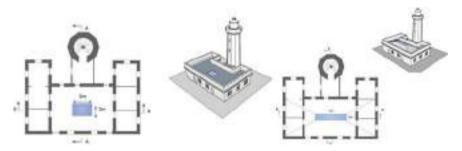
Fig. 5 The new skylight: on the left the simple one; on the right the pavilion skylight
