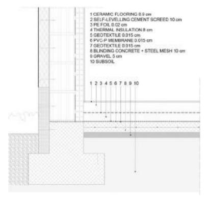
Fig. 3 Detail of a floor structure with continuous radon proof membrane
