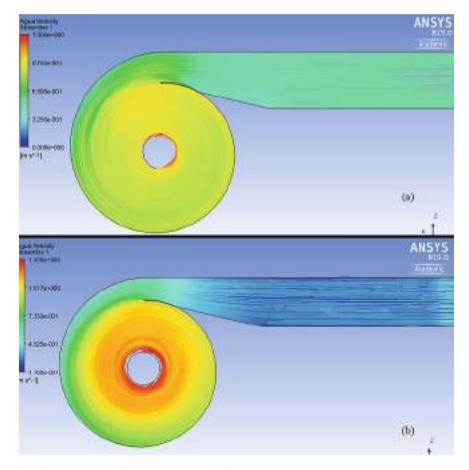
Fig. 6 Streamlines at 35 s. a prototype A and b prototype B
