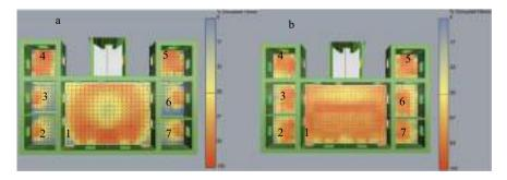
Fig. 7 UDI maps with a with simple skylight (SS) and b with reflective slatted panels (RSP)
