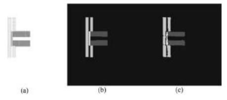
Fig. 6 Visual results of one test example. a Original image, b ground truth label, c the segmented output of the proposed method
