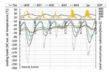
Fig. 3 The data obtained computationally for heat flow response corresponding to the cooling energy load for unvented test case (*Note EXP* results obtained experimentally for validation)
