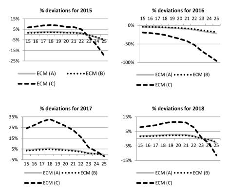
**Fig. 5** Change in the % deviation in energy savings due to the change in CDD base temperature for the different types of ECMs and for the different years under study. Note the different scales for the % deviation
