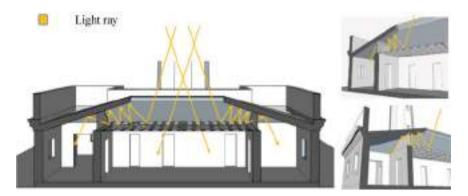
Fig. 6 The light ray simulation inside the restaurant atrium and adjacent rooms
