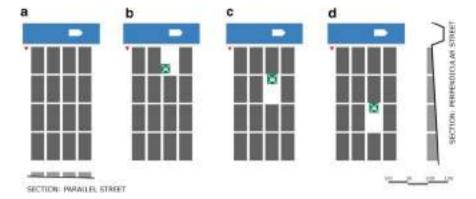
Fig. 1 Typological BEs for evacuation simulation: the blue area is the river (flow direction by the white arrow), which discharges floodwaters in the BE according to the red arrow. Building blocks are grey rectangles. Gathering areas in the square for sheltering strategies are traced by the related signs. Cross-sections are offered (vertical exaggeration of  $10\times$ )
