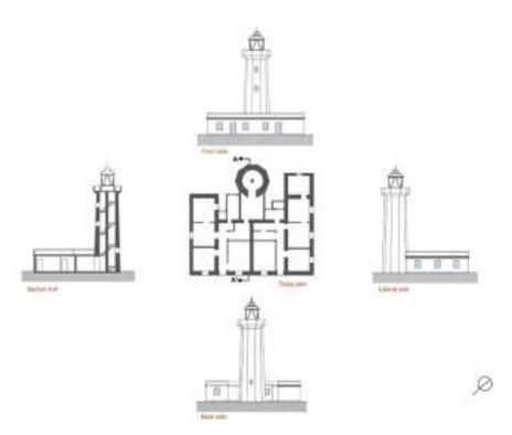
Fig. 3 Geometrical survey of the Capo Murro di Porco Lighthouse
