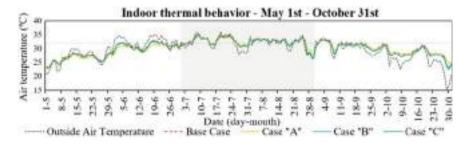
Fig. 7 Chart with the outside air temperature, the  $32\,^{\circ}$ C for indoor "neutral" temperature, and the indoor temperature behavior for all cases
