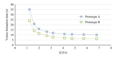
Fig. 5 Vortex formation time comparison between prototype A and prototype B
