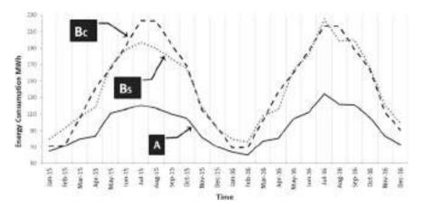
Fig. 2 Estimated energy consumption if no retrofitting is done. Bs is calculated using the computer simulation. Bc is calculated using the CDD method (shown here for base temperature =  $18 \, ^{\circ}$ C)
