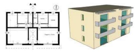
Fig. 1 Representation of the plan type and Schematic three-dimensional model of the building
