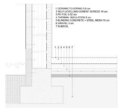
Fig. 2 Detail of basic floor structure without radon-proof techniques
