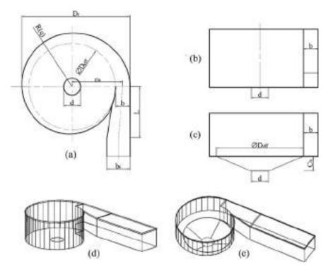
Fig. 1 Components and dimensions of vortex chamber. Top view of vortex chamber  $(\mathbf{a})$ , flat-bottom chamber  $(\mathbf{b})$  conical chamber outlet  $(\mathbf{c})$ , 3D flat-bottom chamber prototype A  $(\mathbf{d})$  and 3D conical chamber outlet prototype B  $(\mathbf{e})$
