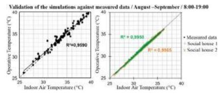
**Fig. 6** Simulation results of two houses ( $R^2 = 0.9958$ ,  $R^2 = 0.9965$ ) contrasted against the data measured in 143 houses ( $R^2 = 0.959$ ) during August and September
