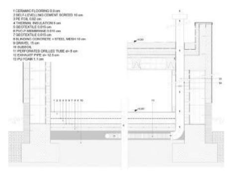
Fig. 4 Natural ventilation of the subfloor gravel layer with perforated pipes and a vertical exhaust pipe
