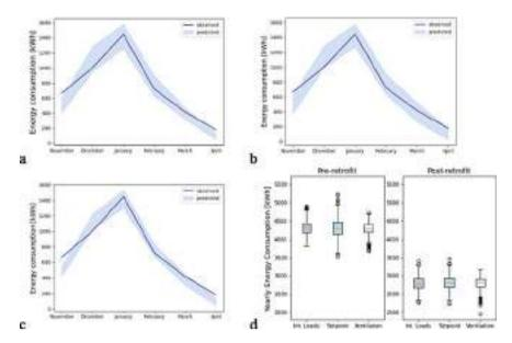
Fig. 3 Monthly EC for the three UAs in pre-retrofit scenario: a IL-UA, b HS-UA and c NV-UA; d box plot of yearly EC in pre- and post-retrofit scenarios
