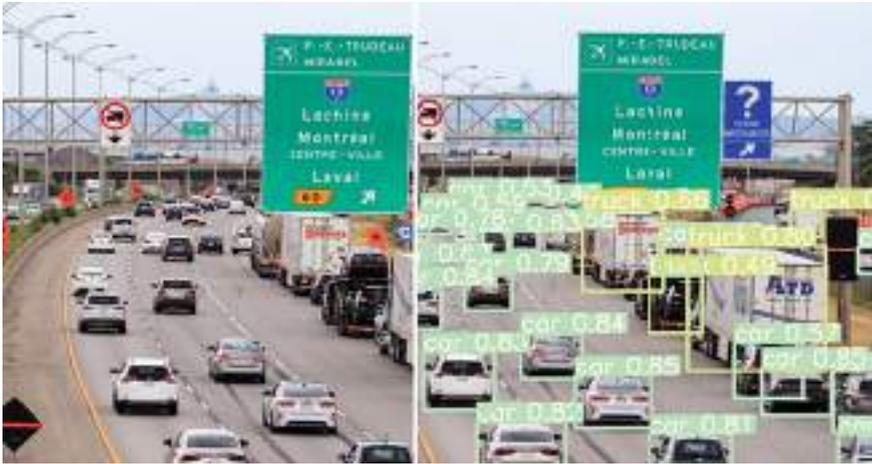
**Fig. 4** Visualization of ground truth bounding boxes for object detection using YOLOv5
