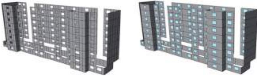
**Fig. 4** Geometrical discretization of facades for concrete (left) and timber panels (right)
