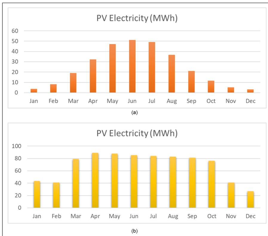
**Figure 10** PV generation potential when installed on (a) roofs and (b) roofs and external walls.
