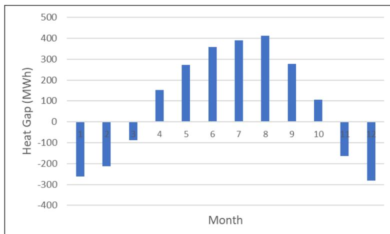
**Figure 13** Gap between heat demand and heat supply by HP.
