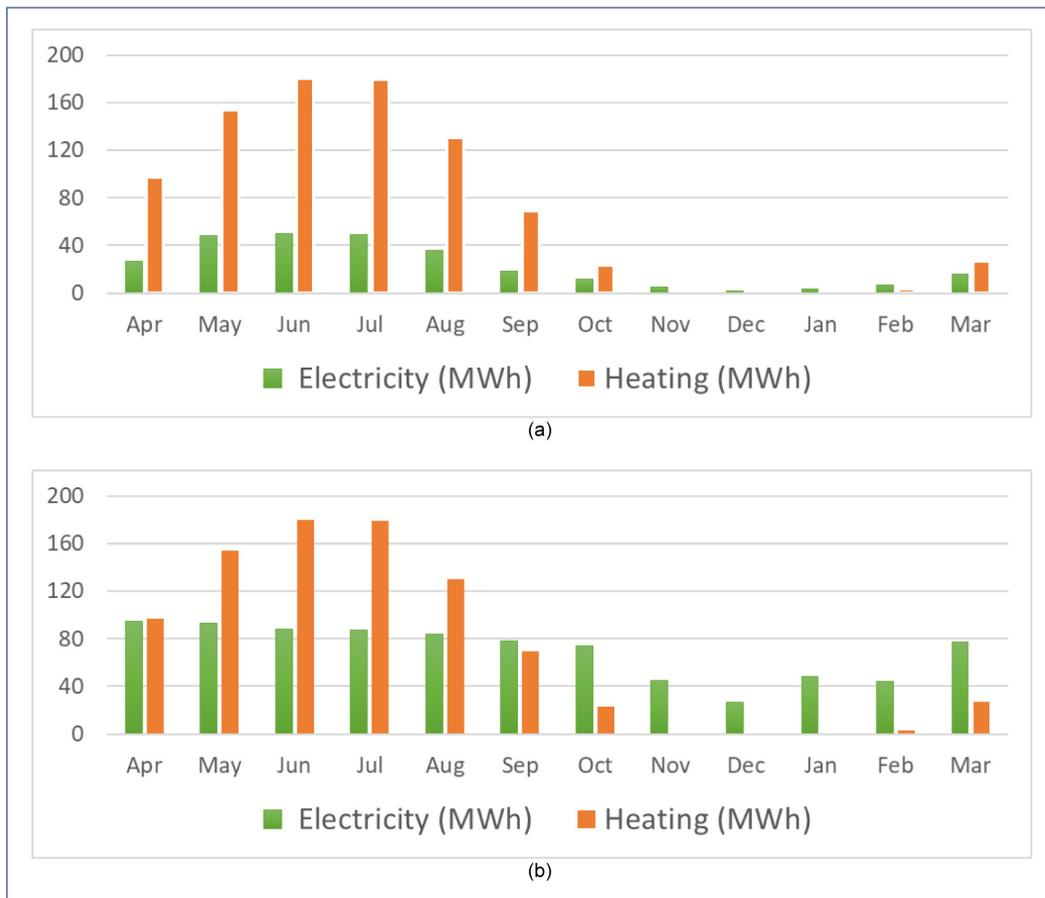
Figure 11 PVT generation potential when installed on (a) roofs and (b) roofs and external walls.
