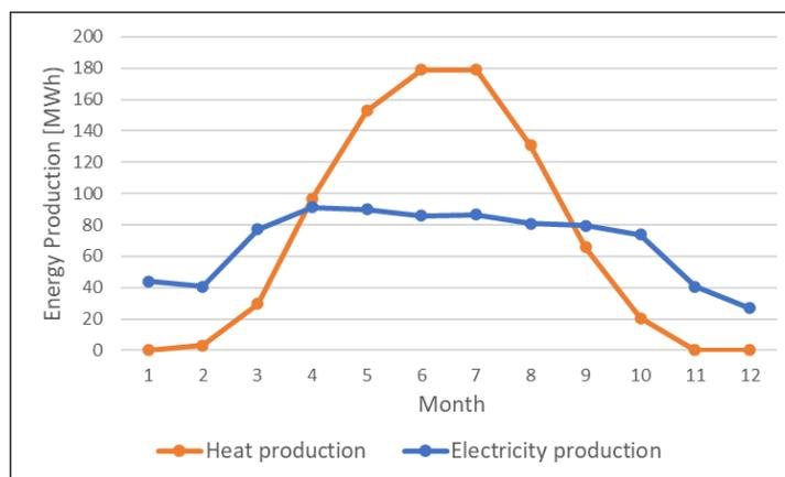
Figure 15 Monthly electricity and heat production of the PVT system.
