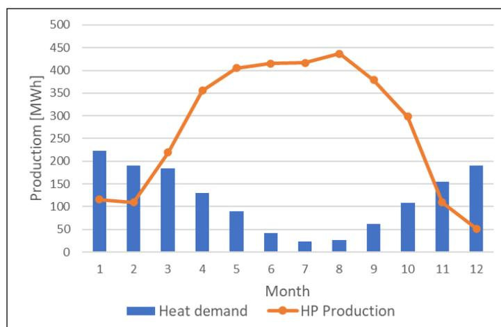
Figure 16 District heat demand and heat pump production with excess heat delivered.
